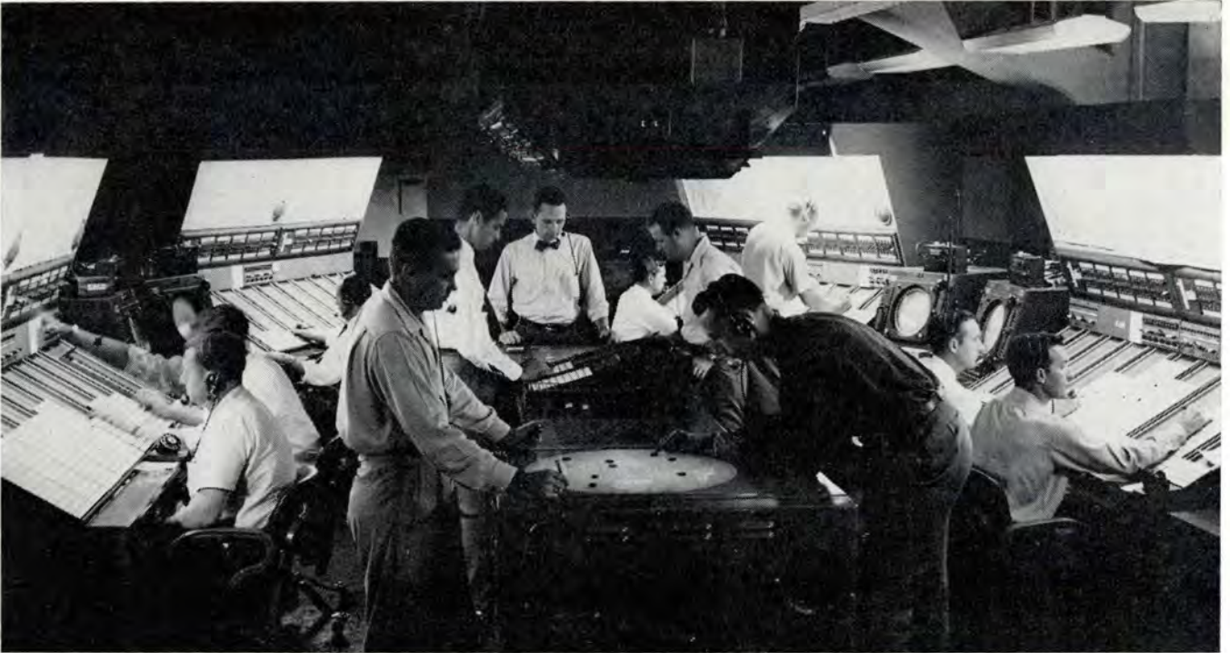
Washington Air Route Traffic Control Center showing controls around horizontal radarscope and manual control board in background.
